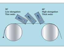
more complex and not generally well understood. Proper nip configuration must consider factors such as: the web path (wrap vs. tangent), blade edge profile, shear (cant) angle, blade
