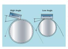
this is usually the only edge that might have an edge bead ("raised edge"), depending on blade profile, etc. Minimizing the effect of this displacement is the key to optimizing
