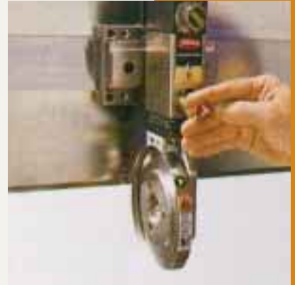
Photo 1: The ability to reverse the cant angle is easily accomplished by rotating the cant-control key in this unit. This allows slitting on the opposite edge of the lower slitter ring. No tools are required.
