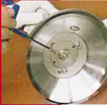
Photo 2: Replacing a slitter blade is best done off-machine. In this example, the retaining screws are recessed, so the retaining ring or blade cannot be ejected if an operator fails to adequately tighten a screw. This is especially important on high-speed slitters, which require an extra-secure, blade-mounting system. This design is not influenced by blade rotations, as is the case with large-diameter, threaded blade-retaining nuts.
