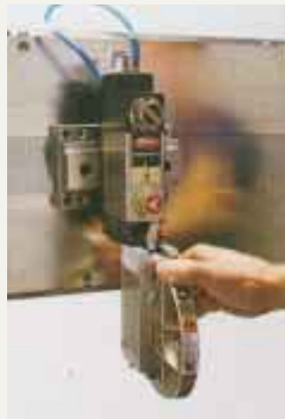
Photo 3: A tool-free removable cartridge makes off-machine blade changing safer. This is especially important where access is awkward or hazardous. Machine downtime is also reduced.
