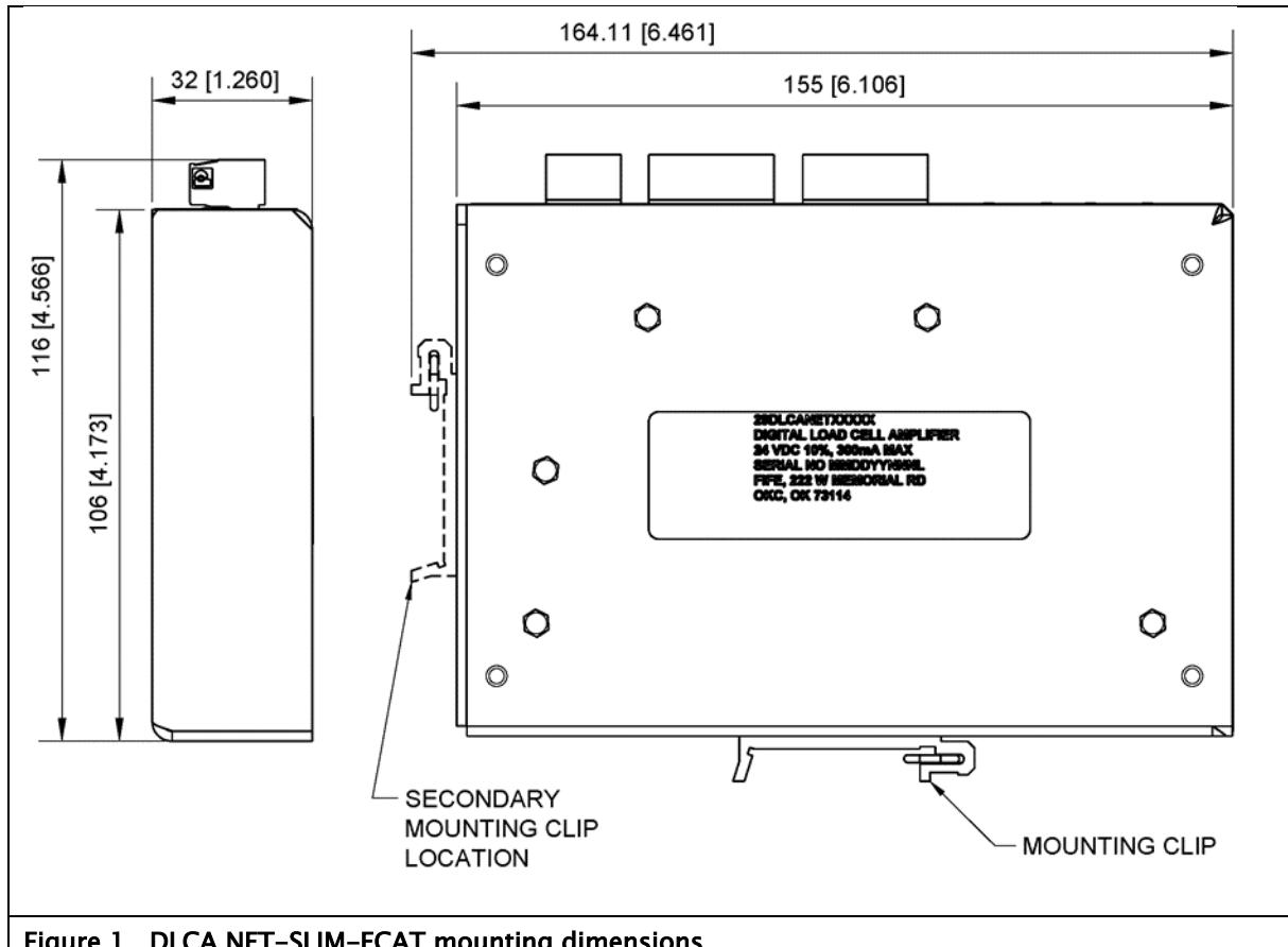
Figure 1. DLCA NET-SLIM-ECAT mounting dimensions
