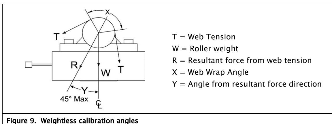
Figure 9. Weightless calibration angles
