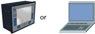
The camera is operated entirely via a D-MAX OI-B or OI-N operator interface, or via a PC-based virtual OI.
