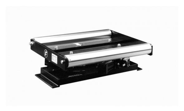
The LRB offset pivot guide is designed for reliable performance using either an electromechanical actuator or hydraulic cylinder as a power source. Constructed with low-friction ball bushings and precision race rod supports, this versatile guide delivers low-maintenance operation for edge, line, or center guiding applications.
