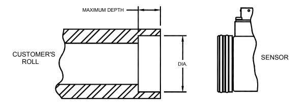
Insert one sensor into each end of a machined tube, and install between machine frames accordingly.
