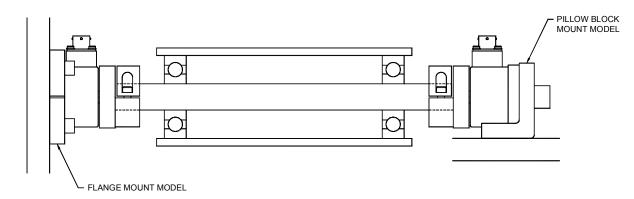
The In-Roll configuration supports the customer's roll assembly (hollow tube) on each side of the machine. Sensors with in-roll couplings are available with all three mounting types.
