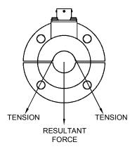
NOTE: If the orientation of the sensor requires the force direction arrow to be pointed opposite the resultant tension force direction, then the black (-S) and the white (+S) sensor leads to the MAGPOWR readout or control terminal block must be reversed.
