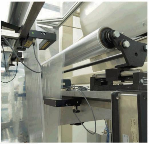
Noven Pharmaceuticals uses a Fife web guide controller with ultrasonic sensor to guide two webs to the sealing nip prior to oven/dryer.
