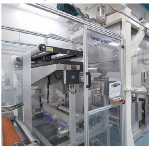
Recent technology investments in converting equipment, including the Fife offset pivot guide with web guide controller, fulfill engineering design concepts as well as the pharmaceutical necessities that are paramount in manufacturing a high quality transdermal delivery system product.
