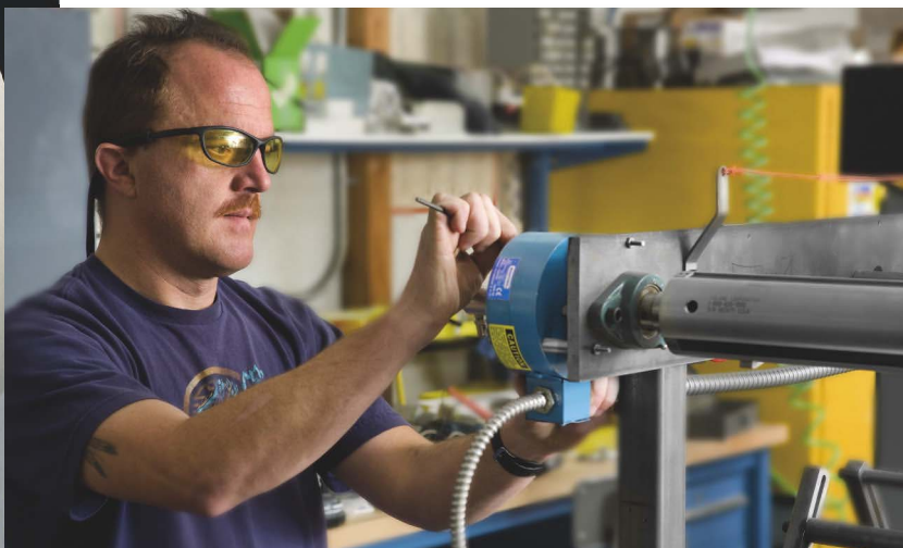
Maintenance technician John Casey adjusts the MAGPOW magnetic-particle brake on one of the Suterra converting lines.
