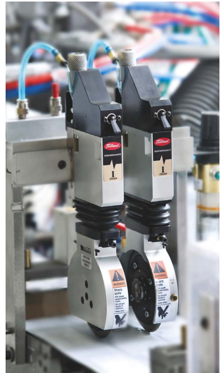
Tidland Class 1 Performance Series knifeholders crush-cut the product laminate into three separate webs.
