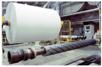
with a spiral design that provides 360° of radial grip and intrinsically equalized load distribution.
