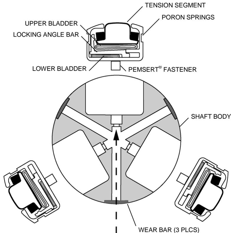
Insert hex wrench through holes in wear bars to access the fasteners that hold trays in place.
