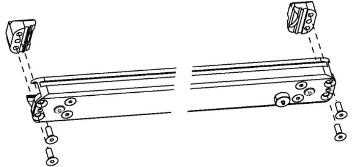
2. Push – and gently pull – on the tension segment strip to slide it out of the tray. Use care not to tear the fragile Poron spring material.
