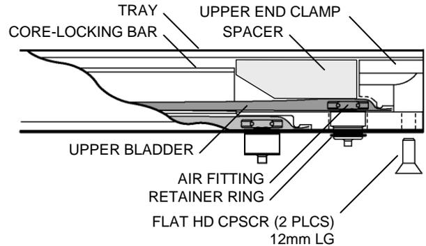
8. Cut other end of the bladder square at a point that lines up at the edges of the screw holes, as shown.
