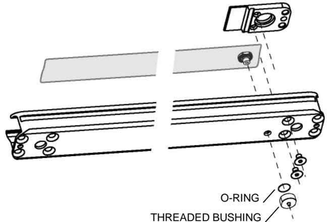
**Note:** Retain the o-ring that is seated in the threaded bushing.
