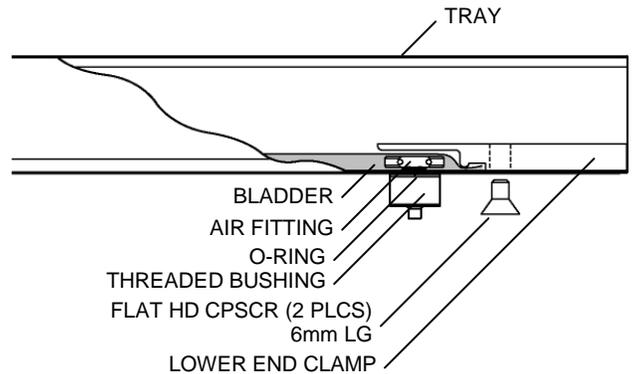
7. Mark the other end of the bladder at a point that lines up just at the edges of the screw holes, as shown, and cut the end of the bladder square.
