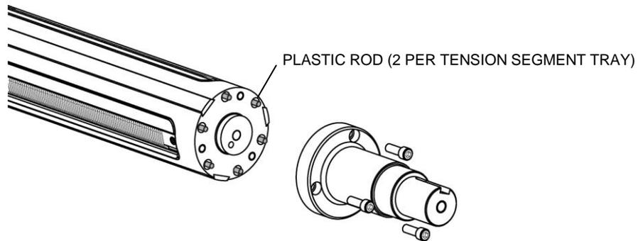
3. Remove the socket head capscrews that secure the tray to the slot. (7/64" hex drive)
