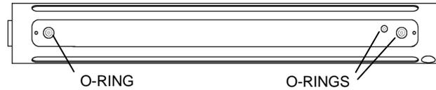
2. Insert the tray in the shaft slot, making sure that fittings on the bottom of the tray align with holes in shaft slot.
