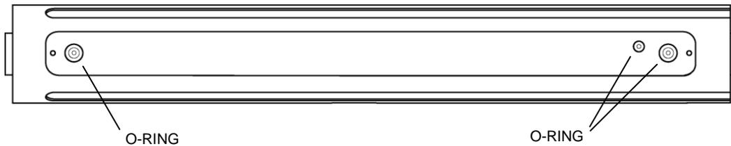
3. Apply a small amount of o-ring lubricant to each o-ring before beginning reassembly.
