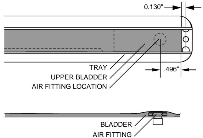
4. Reinstall the bladder in the tray with the air fitting extending through the hole in the lower element end clamp.
