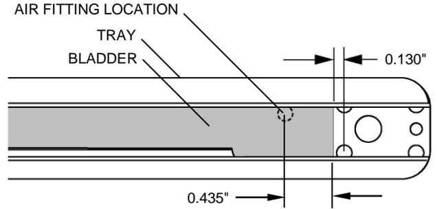
3. Using the Tidland Hole Punch Tool, punch a hole in one wall only of the bladder and insert the air fitting into the bladder.
