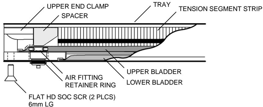
**Before continuing reassembly,** test the bladder for air leaks at 80 psi (5.5 bar) using soapy water at end clamps and air fitting. When inflated, the bladder should cause the tension segments to lift.
