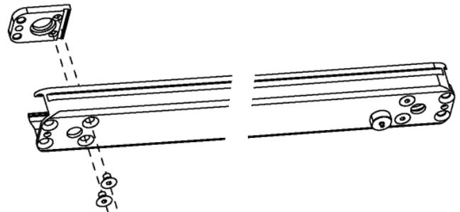
5. Slide the core-locking bar out of the tray.
