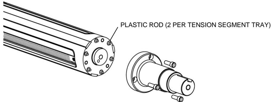
3. Remove the socket head capscrews that secure the tray to the slot. (7/64" hex drive)
