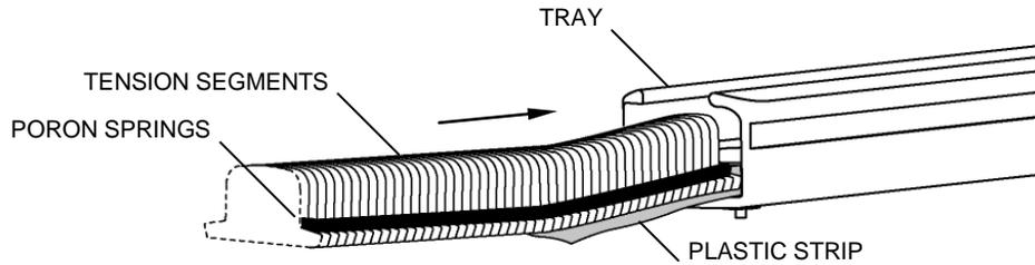
4. When the tension segment strip has been completely loaded into the tray, install the short plastic spacer, in the direction shown below.
