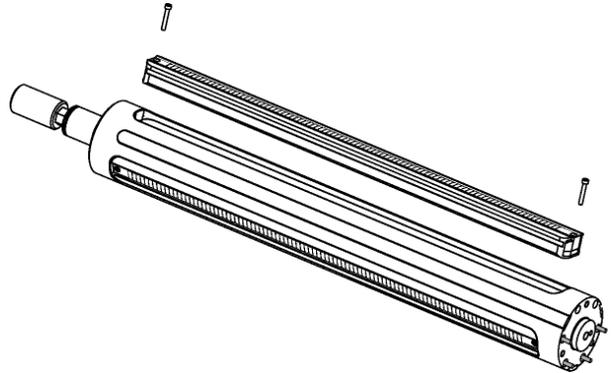
5. Slide the plastic rods into the grooves in the shaft to retain the tray. If they do not slide in easily, press down gently on the tray as the rod goes into the shaft.
