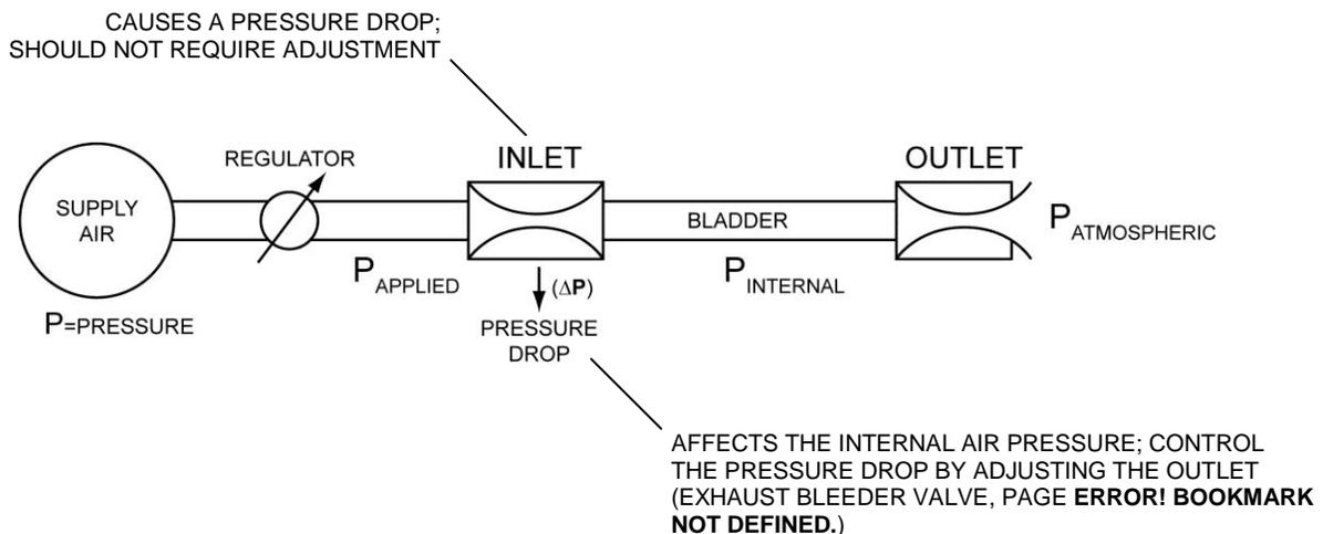
**For the D3 Differential Shaft, this Pressure Control Valve System affects only the upper bladder that controls the tension segment height.**
