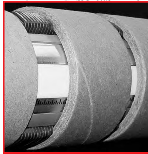
Tension Segments also act as core stops to eliminate lateral roll movement
