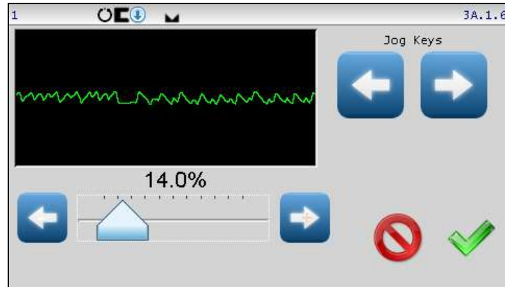
Figure 7. CONTROL PANEL SYSTEM GAIN SETUP SCREEN
