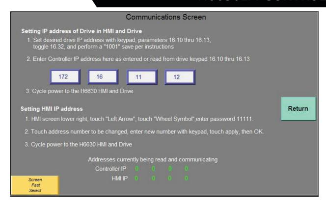
Configuration and calibration are easily accomplished using the HMI. The H6630EM communicates with all common industrial networks and the controller program is provided on a USB device for user back-up and retention. It can communicate with any programmable logic controller that is based on the open international standard, IEC61131-3.
