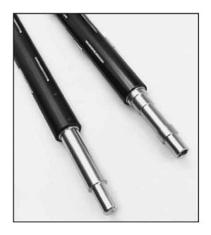
The Series 500 Lug Shaft is designed for light- to heavy-duty applications in 50.8 mm (2 inch) to 152.4 mm (6 inch) ID cores, often used in center unwind and rewind applications with either fiber or steel cores. These reliable shafts are constructed of alloy steel, aluminum, or lightweight, composite materials depending on usage and requirements.
