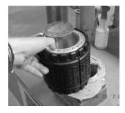
Place solid insert in spool and tire on spacer
