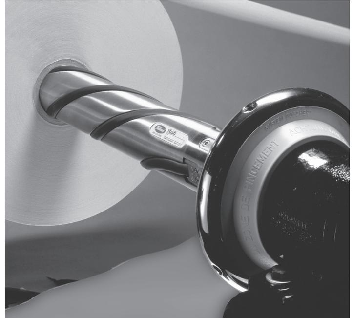
Manual Safety Chucks are available in fixed or sliding designs, with a unique self-closing feature to ensure safe performance even if the operator neglects to close the chuck after loading. An effective load bearing design ensures long life and smooth rotation. Optional replaceable socket inserts and adapters for MAGPOWR global brakes make these chucks suitable for virtually any application.
