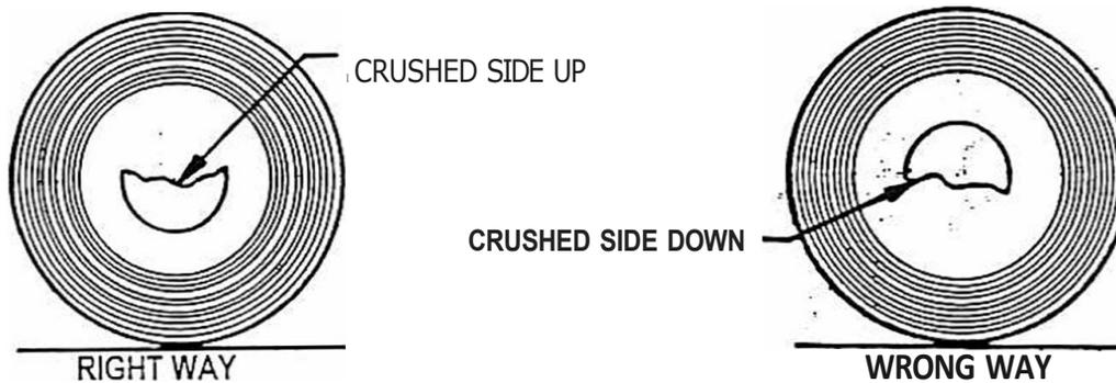
Before the Roll Restorer is engaged in the crushed roll, the roll should be positioned with the crushed side UP as shown above. Also, when aligning the housing and ram assembly with the center of the roll, care should be taken to align the two as close as possible to the same centerline.
