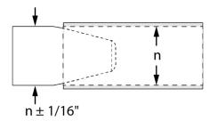
The expander head can be plus or minus 1/16" in outer diameter from the internal diameter of the crushed core original diameter (n).
