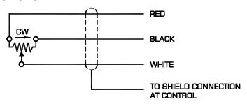
To find the electrical center point of pot rotation, use a digital multimeter type ohm meter to measure from the white wire (wiper), to the red or black wire. Turn the potentiometer shaft until the meter reads  $500\Omega$ .
