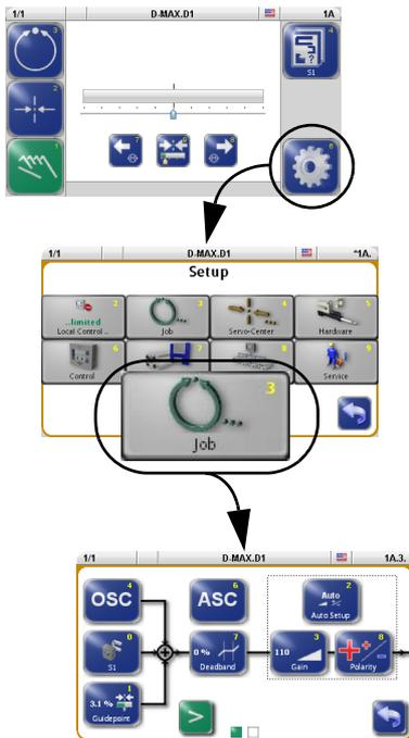
This section is a description of menus that are used to set up the parameters of a job. A similar set of parameters is available for each job in the system. The settings of this job apply to "Automatic" mode.
