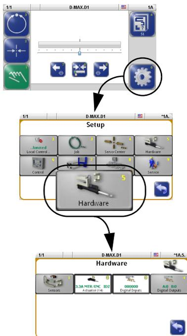
This section contains a description of menus that can be used to view and set up the properties of the connected input and output devices.
