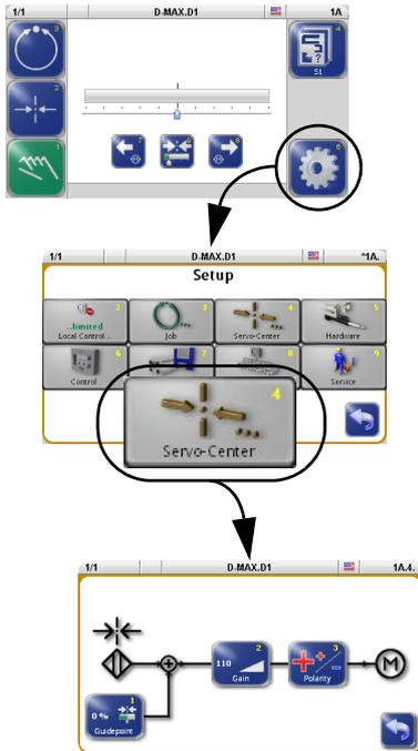
This section describes menus that are used to set up the properties for "Servo-Center" mode.
