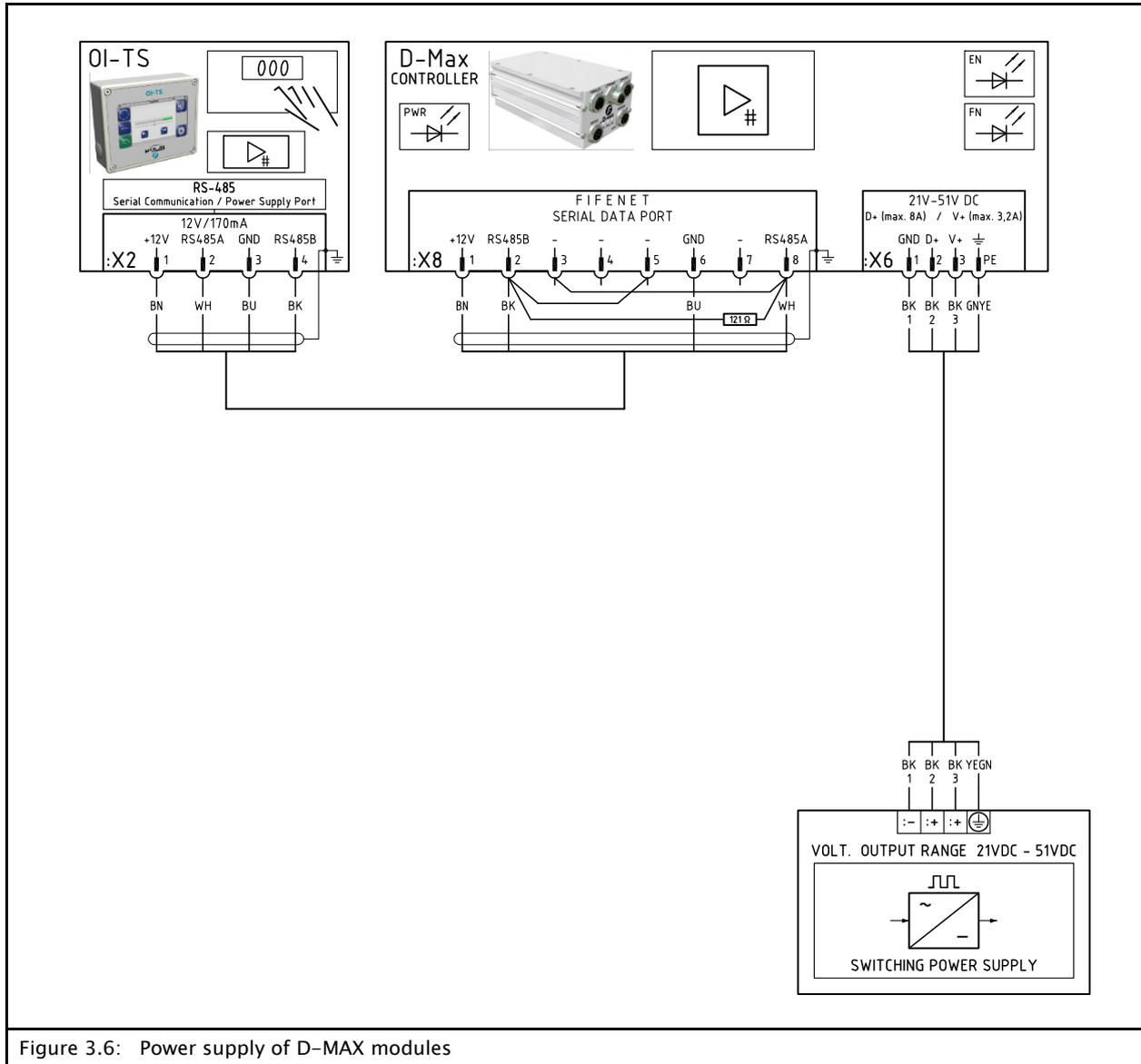
Figure 3.6: Power supply of D-MAX modules
