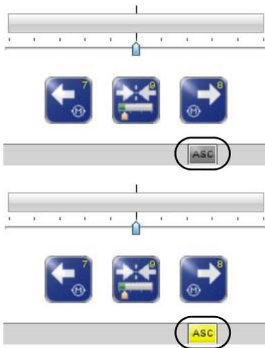
If the D-MAX system is in "Automatic" mode and the ASC parameter is activated, the web is guided as long as it is within the restricted field of view of the sensor. This is indicated by the gray "ASC" icon in the status line.
