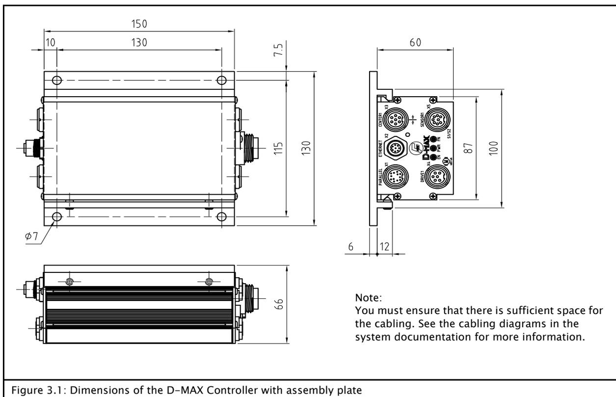
Figure 3.1: Dimensions of the D-MAX Controller with assembly plate
