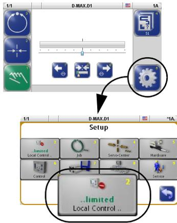
The *Local Control* menu can be used to block control signals which are a hindrance during initial operation or an error search. Control signals can be:
