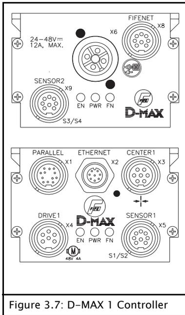
Figure 3.7: D-MAX 1 Controller
