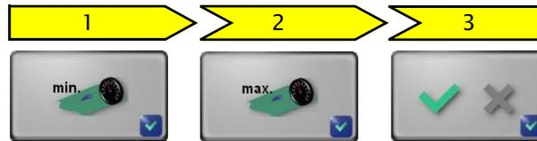
1. The reference value for the minimum web speed must be determined.
