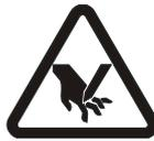
There is a risk of being cut by the web and crushed against the actuator.
