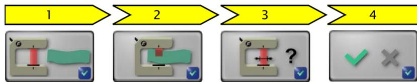
1. The reference value for the uncovered sensor must be determined. To do this, remove the material web completely from the sensor's field of view.
