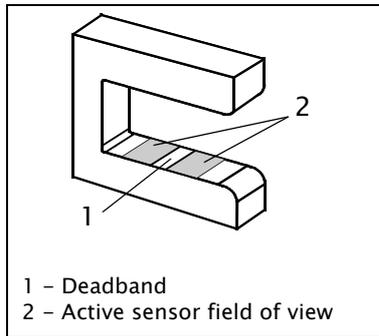
You can use the *Deadband* menu to define an area around the guidepoint inside the sensor's field of view in which guiding is not active in "Automatic" mode.
