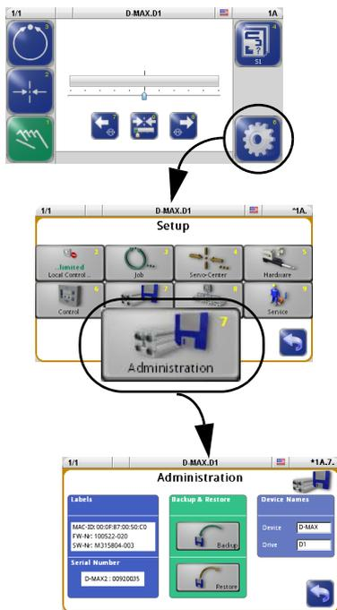
This section includes a list of menus containing information about the D-MAX Controller. This information is required when ordering replacement parts or for service inquiries.
