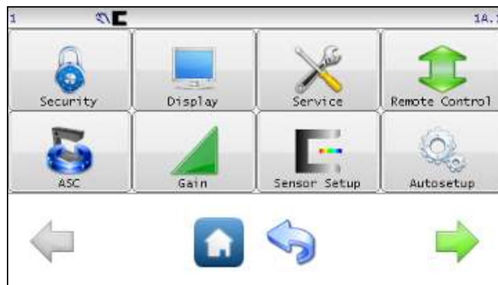
Figure 3. FIFE-500-XL CONTROL PANEL LEVEL 1 SETUP SCREEN
