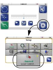
The *Local Control* menu can be used to block control signals which are a hindrance during initial operation or an error search. Control signals can be:
