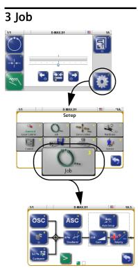
This section is a description of menus that are used to set up the parameters of a job. A similar set of parameters is available for each job in the system. The settings of this job apply to "Automatic" mode.
