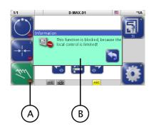
A Keys which are blocked by an active control signal are marked.
