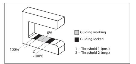
If the D-MAX system is in "Automatic" mode and the ASC parameter is activated, the web is guided as long as it is within the restricted field of view of the sensor. This is indicated by the gray "ASC" icon in the status line.
