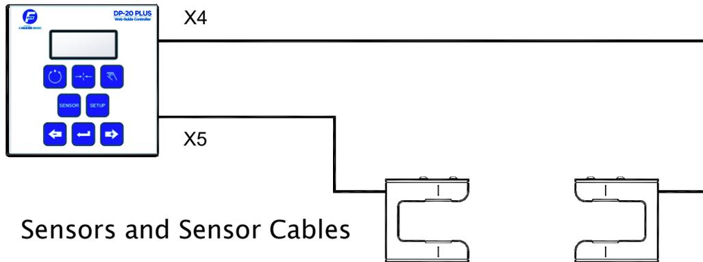
Figure 4 - Center Guiding Setup
