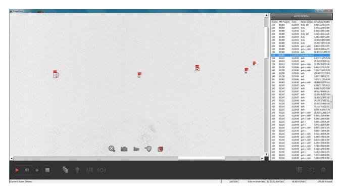
ImageFlow RT achieves this with a one touch system for mode operation and recipe selection. The defects are clearly displayed with context. Rather than displaying a small region of interest that looks like a postal stamp, the operator sees the defect on an image of the complete web. Finally the historical information for that run with a time stamp and location is displayed on a list to the right hand side. The operator simply selects the event and can see the web image at that time.
