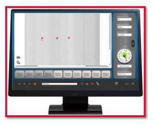
Imageflow supports any number of product recipes, and will store all defect images with the exact location and position.
