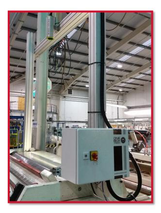
Use the system to count gels and analyse according to a defined area, enabling real time grading of the film.
