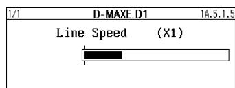
The Line Speed signal that is currently present is shown in the bar graph.
