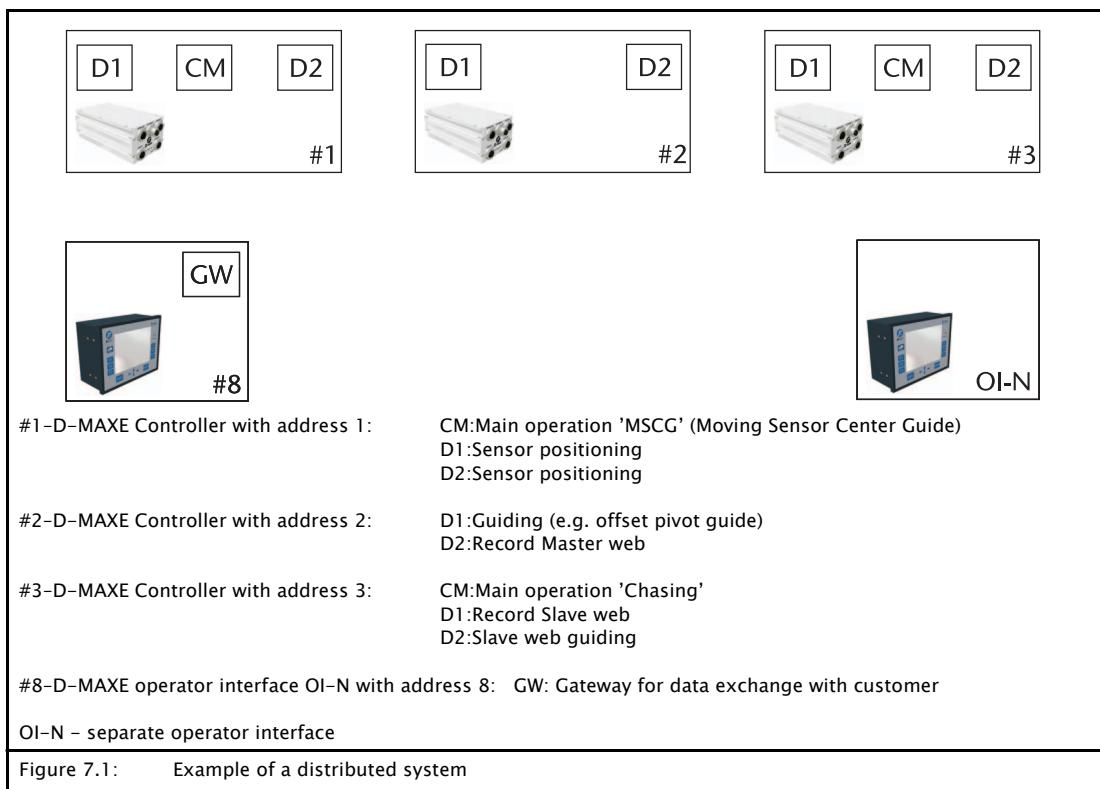
All elements ("devices") present in the distributed system can be selected in operator interface OI-N.
