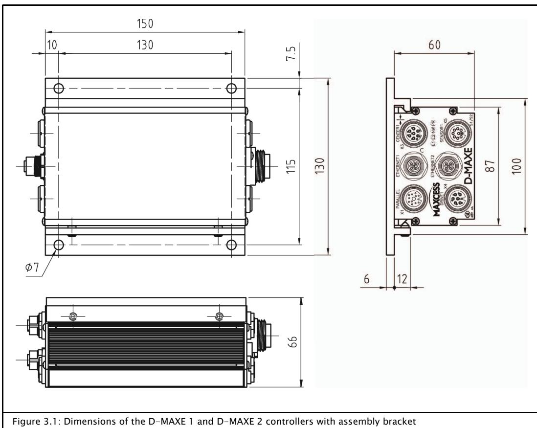
Figure 3.1: Dimensions of the D-MAXE 1 and D-MAXE 2 controllers with assembly bracket
