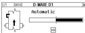
If the D-MAXE system is in "Automatic" mode and the *ASC* parameter is activated, the web is guided as long as it is within the restricted field of view of the sensor. This is indicated by the "ASC" [0010] icon in the display.
