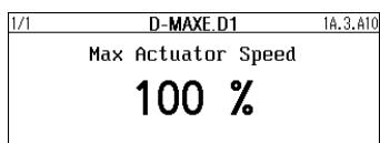
The current setting of the *Max. Actuator Speed* parameter appears.
