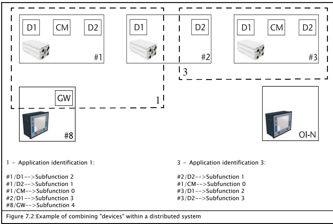
Every "device" inside an application has a subfunction with its menu structure. The **1y.7.5.2 Sub Function** menu gives a unique designation ( $n = 0 \dots 255$ ) to these menu structures.
