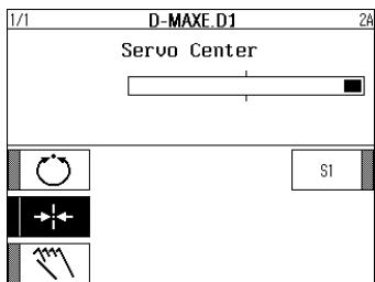
The bar graph identifies the position of the Servo-Center transducer's guidepoint.
