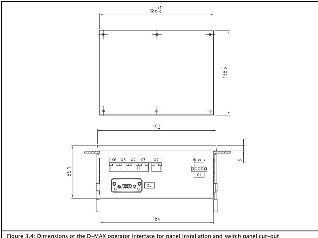
Figure 3.4: Dimensions of the D-MAX operator interface for panel installation and switch panel cut-out
