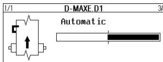
The guidepoint is reset to 0%. The triangle under the bar graph disappears.
