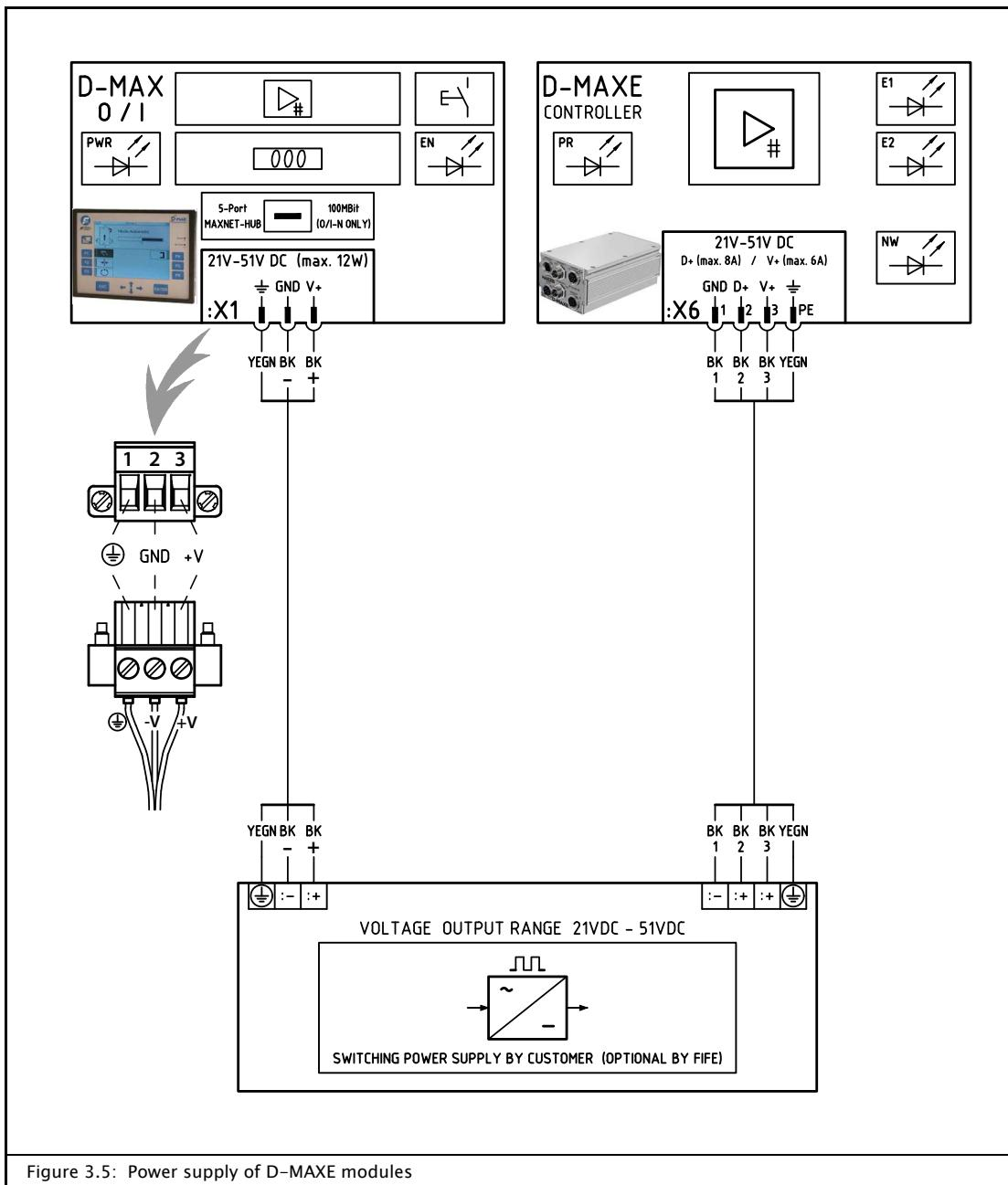
Figure 3.5: Power supply of D-MAXE modules
