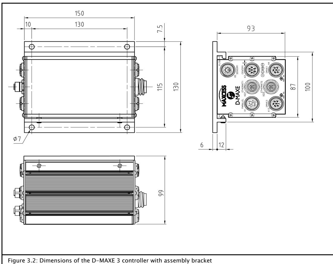
Figure 3.2: Dimensions of the D-MAXE 3 controller with assembly bracket
