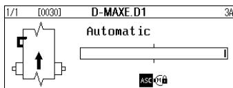
If the web leaves the limited field of view of the sensor, guiding is blocked. This is indicated by the "ASC" and "Motor locked" [0030] icon in the display.
