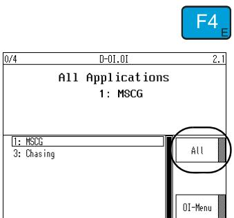
If the "devices" in the network are filtered and a "device" the user is searching for does not appear in the list, filtering can temporarily be turned off with the F4 key (see *Distributed system* on page 7-47 and *Application filter* on page 5-5).
