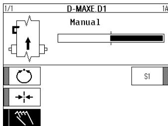
The bar graph identifies the position of the guidepoint of the sensor selected with F4.
