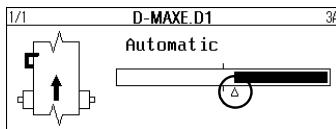
A triangle and guidepoint shift percentage appear under the bar graph at the point to which the guidepoint was moved.
