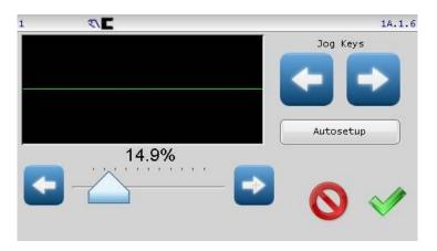
When the gain menu is accessed from Manual mode, the Autosetup button will be shown in one of the following two states, depending on the sensor signal level of the active sensor mode:
