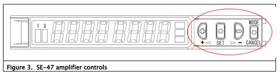
Lift the small cover on the SE-47 amplifier to access the control buttons. Control button labels are shown in [brackets] below.
