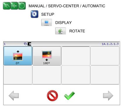
Select the desired screen rotation and press the ACCEPT button to save. The screen will go blank for a moment and restart in the new orientation.
