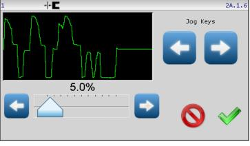
The larger arrow buttons may be used to jog the guide in either direction, if desired.
