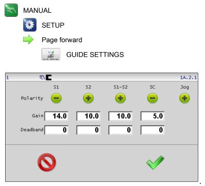
**Polarity** – The polarity buttons display the current polarity settings active for Servo–Center, guiding (each sensor mode), and jog operations. Using these controls polarity can be set manually. To change polarity, touch the desired polarity button to toggle between positive and negative settings.
