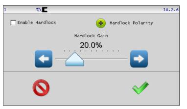
Enable Hardlock Check this box to turn the hard lock feature on.Hardlock Polarity Sets the hard lock correction polarity.Hardlock Gain Sets the hard lock control loop gain. This can be changed with the slider control or with the arrow buttons for finer control.
