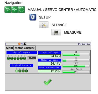
Voltages that are out of range will be marked with a red background as shown below. Notice that the voltage error icon is visible on the status bar. Since voltages are monitored at all times, the status bar can indicate this error regardless of which screen is active.
