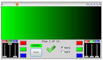
**Test** The Test button cycles through a sequence of gradient settings which would most likely identify hardware related signal issues.
