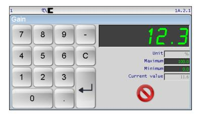
New values are entered using the numeric keypad buttons. Entry format similar to data entry using a calculator where new values appear on the right and shift existing data left. The exception to this is when the first button is pressed the displayed value is cleared first.
