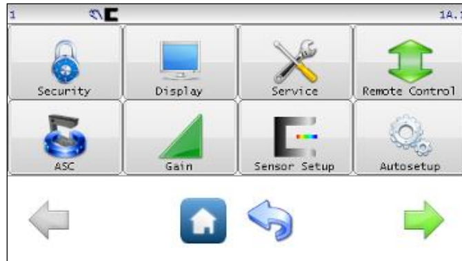
Figure 3 FIFE-500 CONTROL PANEL LEVEL 1 SETUP SCREEN
