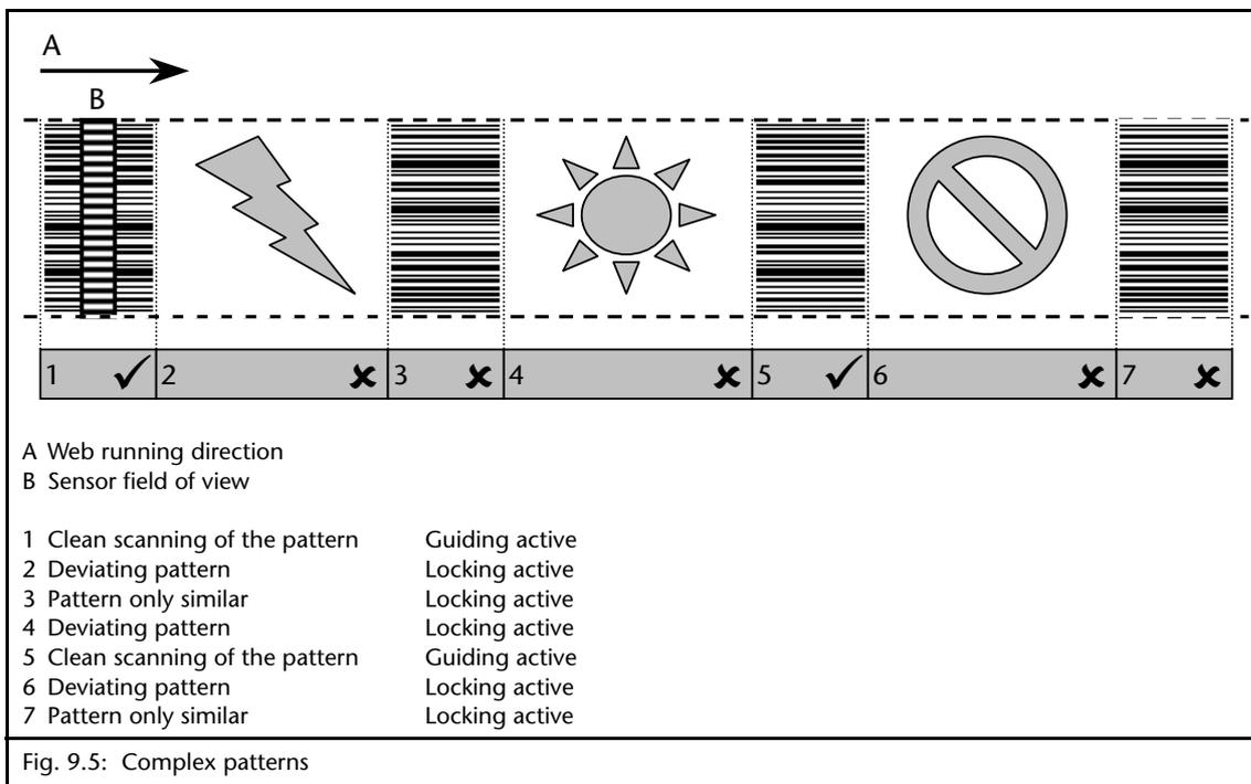
The SE-46 sensor detects a valid position information item (1 and 5), at places along the continuous material web where precisely the calibrated pattern reappears. Other patterns (2, 4 and 6) and other similar patterns as well (3 and 7) are ignored by the sensor and guiding is locked.
