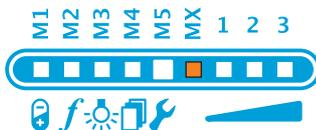
If the calibration failed, lighting is turned off and the message "Calibration invalid" appears in the LED display of the sensor. Sensor calibration must be repeated with better adapted parameters and ambient conditions.
