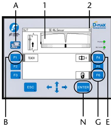
All control functions required for normal operation of the SE-46 sensor are available on the top level of the D-MAX operator interface:
