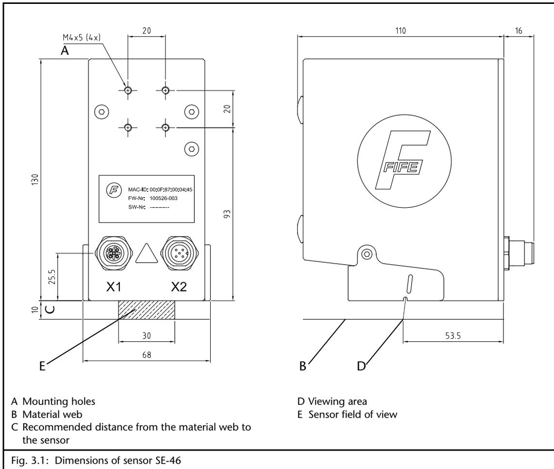
Fig. 3.1: Dimensions of sensor SE-46
