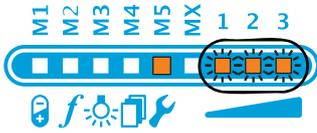
LEDs 1, 2 and 3 flash. Sensor SE-46 sends 10mA to both signal outputs.
