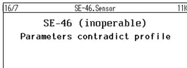
If the parameters for scan frequency or type of illumination are changed, the error message **Parameters contradict profile** appears in the display of the D-MAX operator interface.
