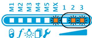
The LEDs of the current setting of the *Profile Switching activated ?* parameter are flashing.
