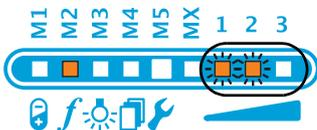
The LED or LEDs of the current setting for the *Scan Frequency* parameter is/are flashing.
