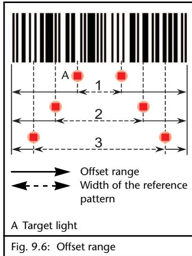
During the calibration process, the user can use the arrow keys to determine which area of the pattern will be saved in the sensor field of view as a reference. This setting indirectly affects the size of the offset range. The greater the width of the selected reference pattern (example 3 - Fig 9.6), the more reliably the pattern can be recognised and the smaller the offset range of the material web.
