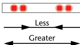
The size of the active area is represented in the target light by lit LEDs.
