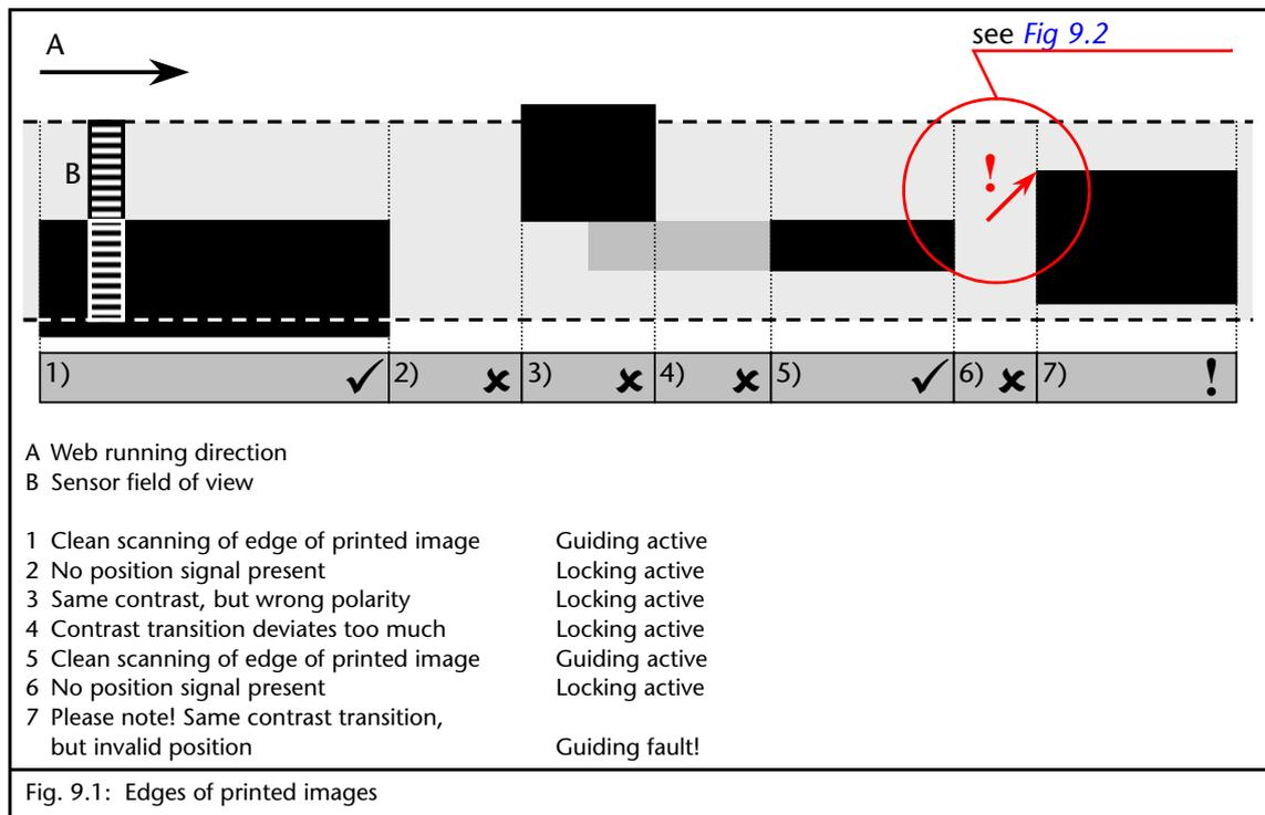
The SE-46 sensor detects a valid position information item (1 and 5) at each of the positions on the continuous material web where the black/white contrast in the field of view is the same as the previously calibrated reference. Reverse contrast transitions (3) and transitions with contrasts of fluctuating intensity (4) are ignored by the sensor and will lock guiding.
