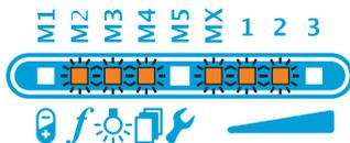
If the parameters for scan frequency or type of illumination are changed after a successful calibration, the operation state error message also appears in the LED display "Calibration invalid".
