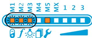
LEDs M1, M2 and M3 flash. Sensor SE-46 sends 0mA to both signal outputs.
