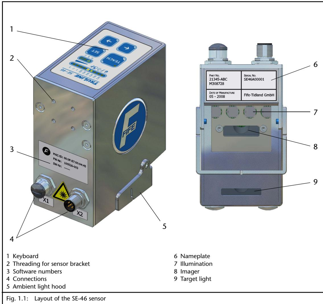
A target light (9 - Fig. 1.1) makes it possible to display detected positions on the material web while operation continues. The distance between the target light and the viewing area is 45 mm (see also A in Fig. 1.2, page 1-3).
