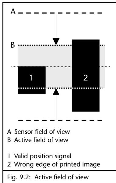
After sections without a position signal (6), the sensor is sensitive to other edges of printed images (7). When the edge of printed image is offset in the field of view, the sensor recognises this contrast transition as valid, resulting in a guiding fault.
