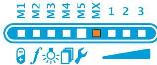
The sensor is reset to the last valid calibration and switches back to normal operation. The target light points at the position of the reference if it is in the field of view.
