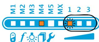
The LED or LEDs of the current setting for the *active profile* parameter is/are flashing.
