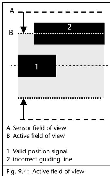
In sections without position signal (9 - Fig 9.3) the sensor is sensitive to other guiding lines. If a guiding line is offset in the field of view, the sensor will detect the wrong line as valid, which will interfere with guiding.
