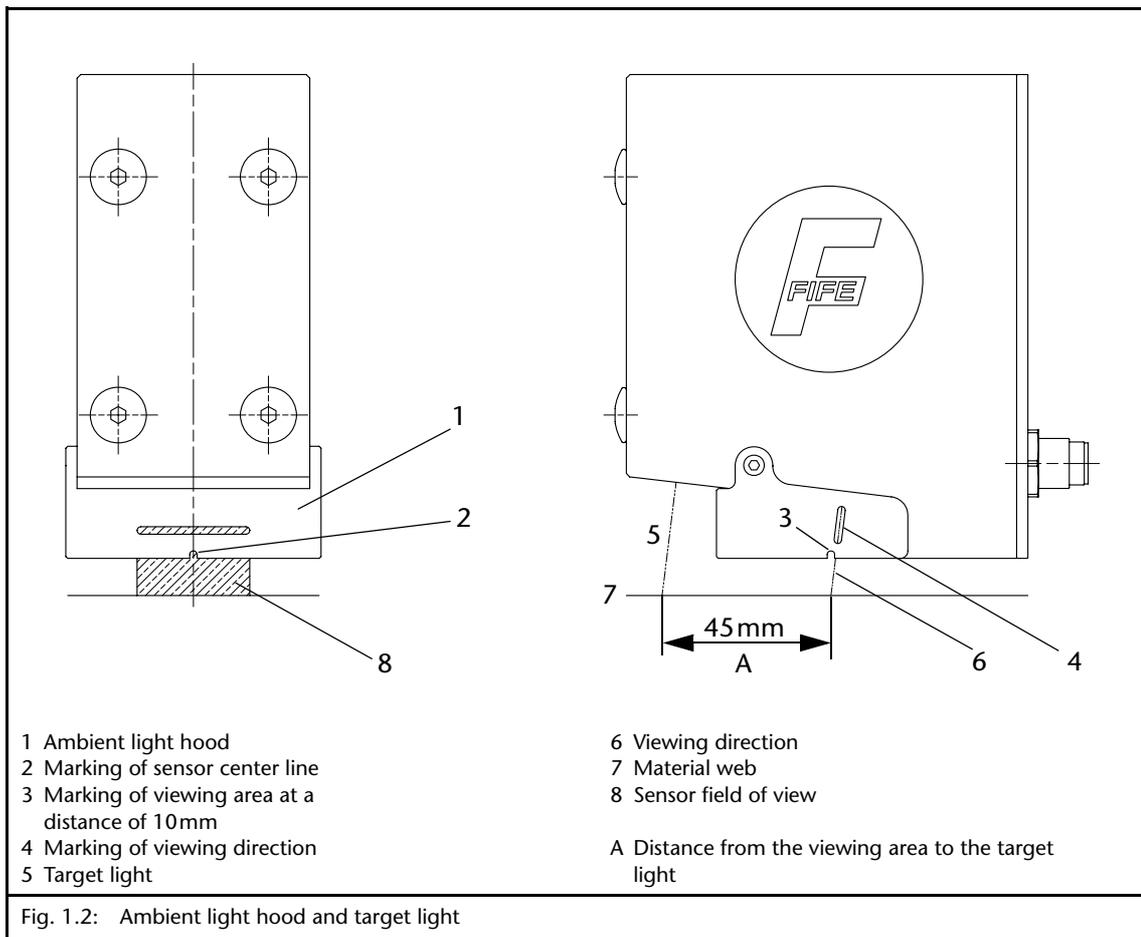
The notch in the front (2) of the ambient light hood identifies the center of the sensor field of view. When the distance between the sensor and material web (7) is 10mm, the notch in the side (3) of the ambient light hood is located exactly above the viewing area. The side slots (4) in the ambient light hood indicate the viewing direction (6) independently of the distance from the sensor to the material web.
