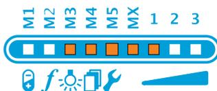
If the D-MAX operator interface is in a menu that is not present in the control tree of the sensor, that will be indicated accordingly in the sensor's LED display and the sensor keyboard will be locked.
