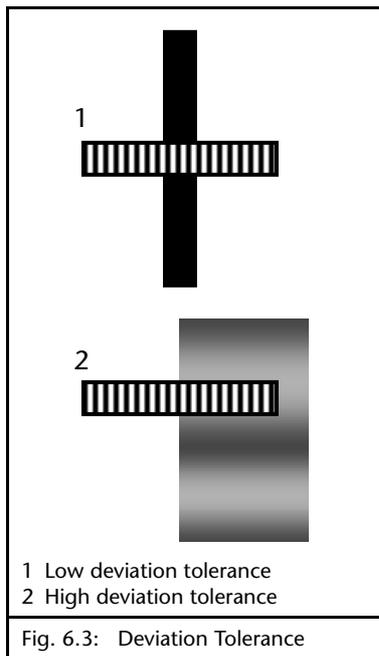
A low deviation tolerance (example 1 in [Fig 6.3](#)) requires a very high match level to the template of the calibrated reference. A low deviation tolerance (example 2) permits greater deviations in brightness or colour, but is also more prone to errors when evaluating similar position marks. This can result in loss of the control point. The recommended setting is "Medium" (see table [Deviation Tolerance](#), page 7-2).
