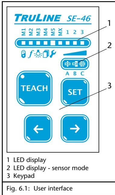
Fig. 6.1 shows the layout of the SE-46 sensor user interface. The sensor has four keys and two LED displays.
