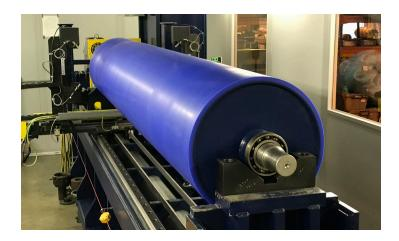
to improve mechanical properties and abrasion resistance. The heat aging properties are substantially better than other competitive abrasion resistant coverings for the general industrial roll market.
