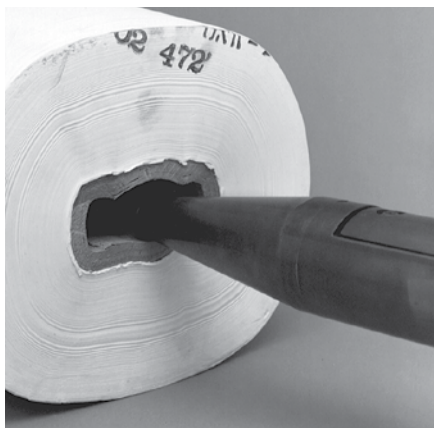
The Mark I Roll Saver is inserted with the pressure plate against the core crush area.
