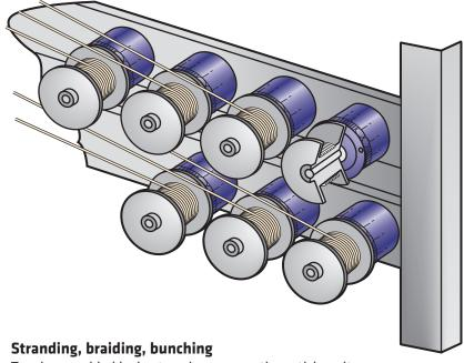
Tension provided by hysteresis or magnetic particle unit
