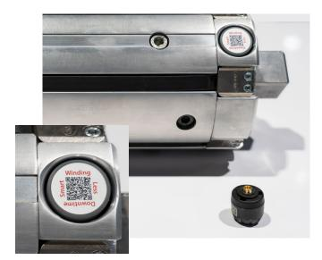
Simply punch the ends of the air bladder and install air fittings (just as would be done during a bladder change) then install a PressureMax wireless sensor in place of the plug. Finally, install a PressureMax Receiver unit to pair with up to (8) shafts, and to display data and alerts in real time.
