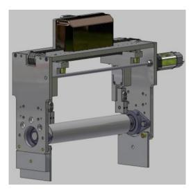
Kit for drop-in mounting between OEM frames (see table) 1x 0.75" dowel pin on rear side aligned to 1x 3/8" thread hole on front side 2x 1.25" spacers and hardware for front side Defined drilling area for adding 2nd front side mounting hole
