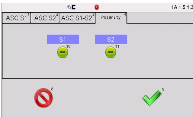
**Polarity:** Used to set the polarities of each sensor signal during ASC processing. The original sensor polarities multiplied by the polarities set here, and then compared it with the ASC threshold value. If it is in the range of ASC threshold value, ASC can be triggered after the Delay ON time when ASC state is on.
