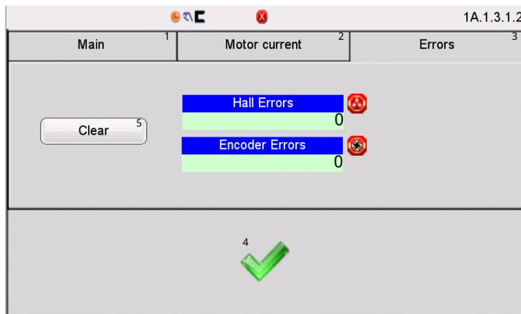
The “Errors” tab displays hall error and encoder error,if an error occurs, the corresponding value will be 1 .
