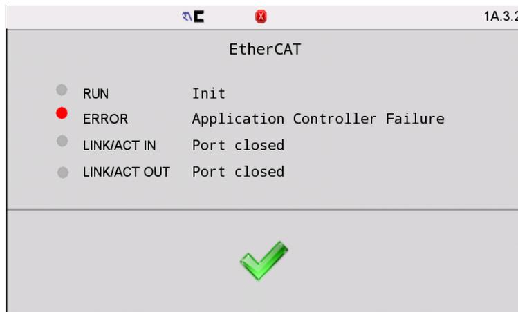
**RUN:** The RUN indicator shall show the status of the EtherCAT Statemachine.
