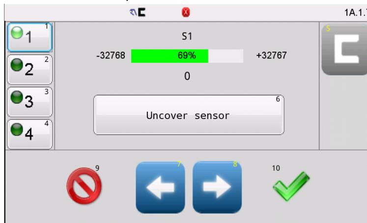
Move the web material completely out of the sensor field of view and press the UNCOVER SENSOR button.
