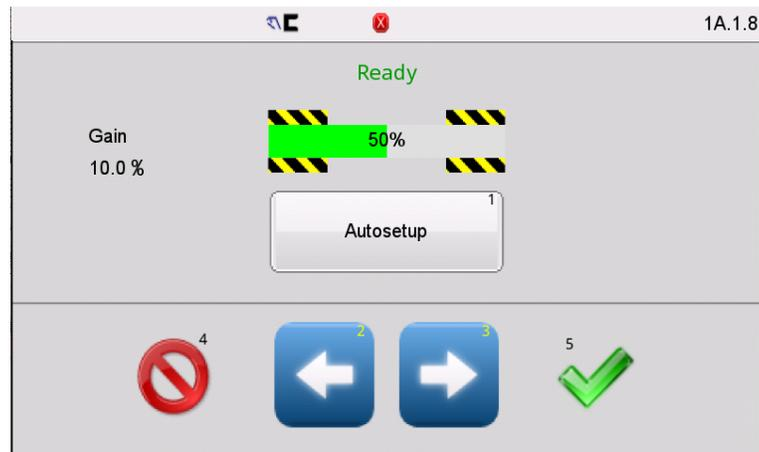
Press the Autosetup button to start. The guide will move a short distance as it completes the auto setup process. Successful completion is indicated by the message shown below.
