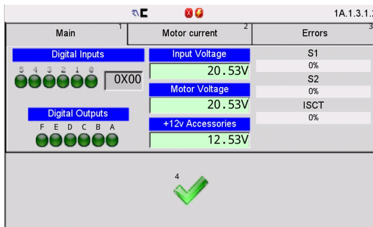
Notice that the voltage error icon is visible on the status bar. Since voltages are monitored at all times, the status bar can indicate this error regardless of which screen is active.
