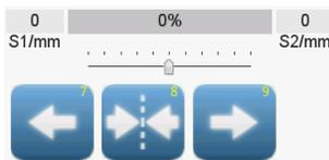
**GUIDE POINT CONTROL** Use the two arrow buttons to adjust the System Guide Point while in Automatic Mode or Manual Mode. Use the center button to reset the System Guide Point to the default value, which is 50% of the sensor bandwidth. The slider control indicates the guide point position.
