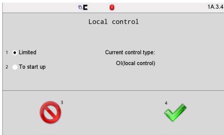
OI operation is limited when connected to remote communications such as Modbus TCP, PROFINET, EtherCAT, CC-LINK IEF Basic. If you need to view or modify settings via OI, select **To start up**, you can have local control for a limited period of 5 minutes.
