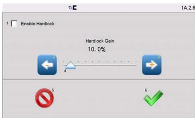
This menu is used to set up parameters to ensure that the position of the drive is actively held when switching into the MANUAL operation mode.
