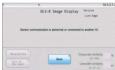
When the DLS-8 communication is disrupted or connected to another Operator Interface (OI), the sensor interface will indicate a communication issue or connection conflict.
