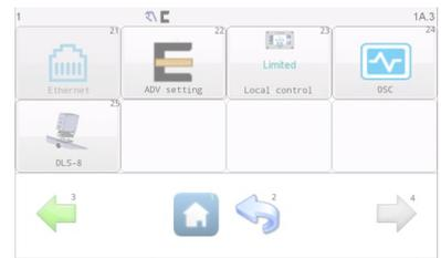
This menu is used to calibrate the gain and polarity of the SmartDrive Actuator (5000,7500&10000N) automatically.
