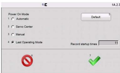
This menu controls the Power On mode for the SmartDrive Actuator (5000,7500&10000N).
