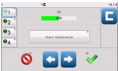
This menu is used to calibrate the settings for the sensors to the properties of the web material.
