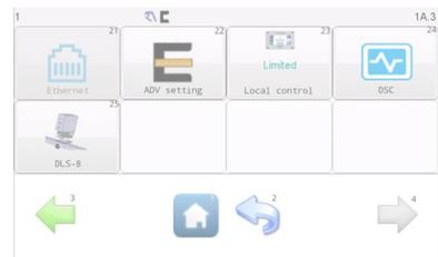
This menu is used to configure authorizations related to operation of the SmartDrive Actuator.
