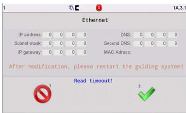
This menu is used to view and configure the Ethernet parameters if the SmartDrive Actuator (5000,7500&10000N) is networked.
