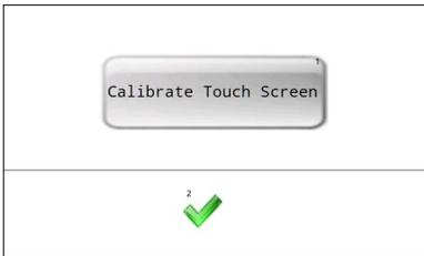
This menu is used to recalibrate the accuracy of the touch screen. This is only necessary if button reactions appear to be out of sync with the displayed button locations.
