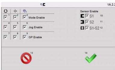
This menu provides elements for the basic setting to operate the SmartDrive Actuator (5000,7500&10000N).
