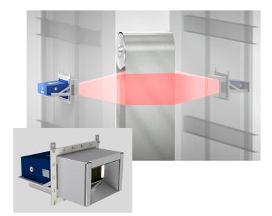
of the metal strip. Furnace windows with non-conductive thermal insulation and mounting flanges are provided, which completely seal the furnace openings and protect the sensors from being damaged by extreme temperatures, contaminants, and contact with the strip. The windows can also be adapted to pre-installed assembly flanges, making it easy to upgrade to higher reliability radar sensor technology without requiring significant mechanical modifications to the furnace.
